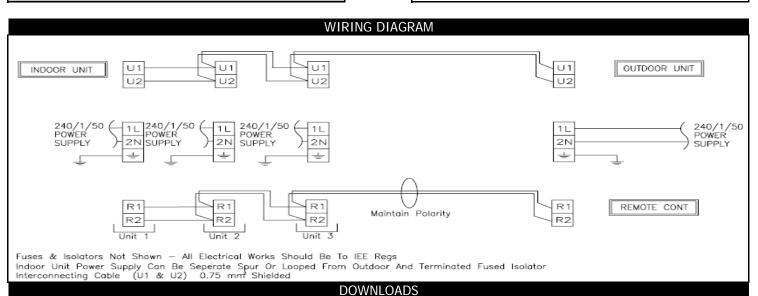
Indoor Unit Model SPW 3:1 Inverter 185 H Outdoor Unit Model
